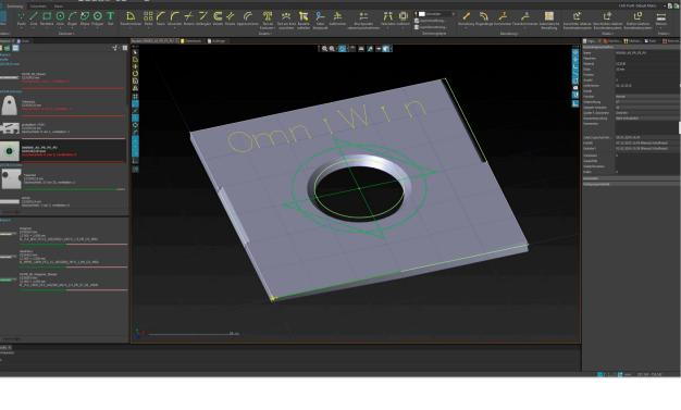
Define standard parts using numerous parameterisable macros and drawing functions for geometric shapes and labels. Use absolute and relative as well as orthogonal and polar coordinates. Convert text objects into closed contours and/or line contours or align them to circular arcs.
