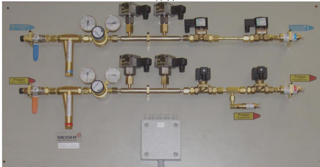
Gas supply panel
